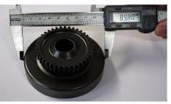
Inner diameter of clutch drum Maximum = 84,90 mm
