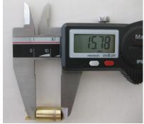
Atomizer, dimension of cutaway: 6,00 +/- 0,15 mm
