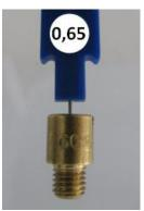
Idle emulsion tube Idle emulsion tube has to be stamped with 45. Plug gauge 0,50 may not enter the central bore. (use jet gauge set Rotax part no. 281 920)
