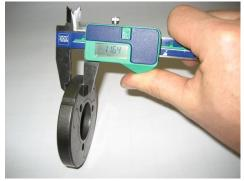
Thickness of clutch shoe Minimum = 24,10 mm
