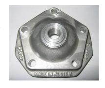
Height of combustion chamber insert has to be 28,80 mm +/- 0,2 mm (H).
