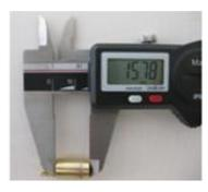
Atomizer, dimension of cutaway: 5,8 +/- 0,3 mm
