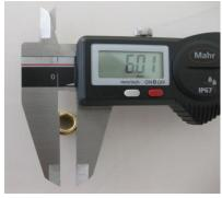
Atomizer, diameter of cross bore: 4,05 +/- 0,15 mm
