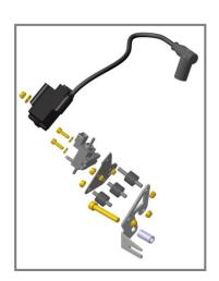
At the mounting versions as shown in the left illustrations, the ground cable of the cable harness has to be connected to the lower rubber buffer of the support plate.
