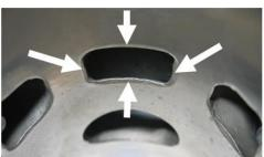
Cylinders marked 223 993, 223 994 and 613 933 the upper edge of the central boost port may show factory machining.
