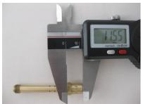
Top bore diameter 2,60 +/- 0,15 mm (measured 2 mm inside)
