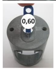
Vertical bore of carburetor insert Plug gauge 0,90 may not enter into bore (use jet gauge set Rotax part no. 281 920).
