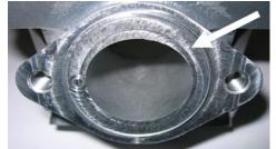
The top edge of the exhaust port may show either just a cast finish surface (left picture) or signs of a CNC machining (central picture) or signs of CNC machining in combination with signs of manual grinding (right picture).
