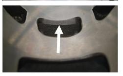
The flange for the exhaust socket may show either cast finish or machined surface.
