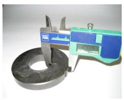
Outer diameter of clutch drum Minimum = 89.50 mm
