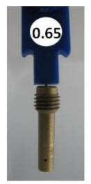
Plug gauge 0,65 mm may not enter one of the 4 cross bores (use jet gauge set Rotax part no. 281 920).
