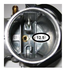
Angular bore of carburetor insert Plug gauge 0,60 may not enter the bore (use jet gauge set Rotax part no. 281 920).
