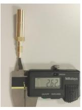
Idle jet Idle jet has to be stamped with 60. Plug gauge 0,65 mm may not enter the bore (use jet gauge set Rotax part no. 281 920).
