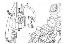
Mounting the ignition coil on the optional bracket (Rotax part no. 651 055) to the clutch cover is an allowed option.
