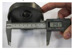
Height of clutch drum with sprocket/primary gear
