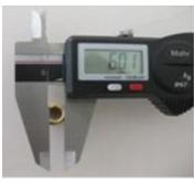
Atomizer, dimension of cross bore: 5,0 +/- 0,15 mm
