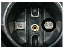
Angular bore of carburetor insert Plug gauge 0,60 may not enter the bore (use jet gauge set Rotax part no. 281 920).
