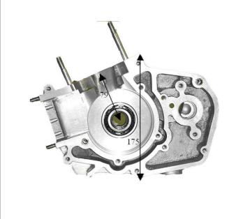
Complete weight = Kg 2,230 Tolerance= ± gr100
