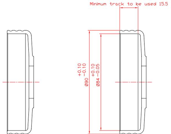
*The complete friction material surface of the clutch rotor must always work into the drum track surface of 15.5 mm (12.5 mm in Super KF with the clutch according to technical drawing No. 17).*
