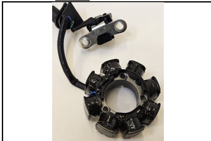
C15-2) Stator - demontert Stator - dismounted
