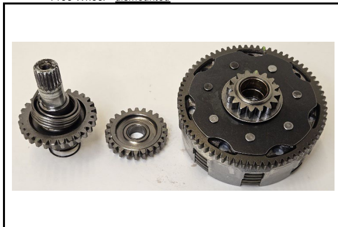
C16-2) Frihjul - demontert Free Wheel - dismounted
