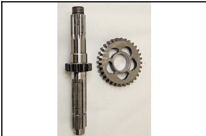
F12-3) Tannjul #1 Sett forfra Gears #1 – Front view
