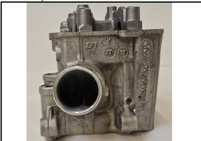
C8-3) Topplukk sett fra insugssiden Bare cylinderhead seen from intake side
