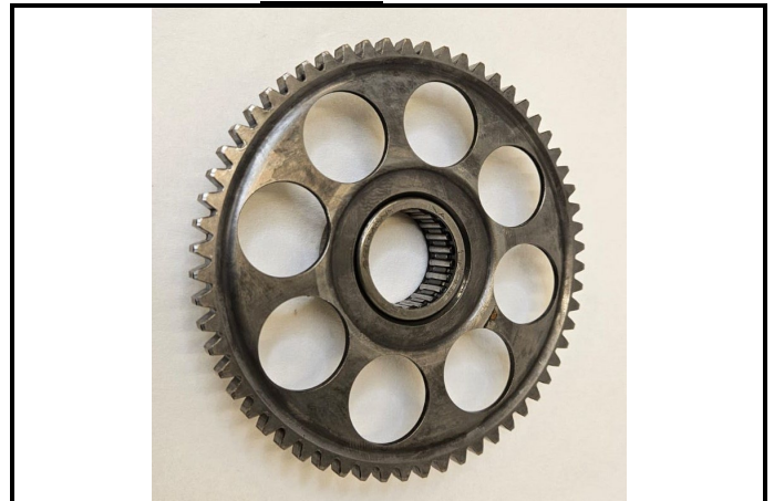
C16-2) Frihjul - demontert Free Wheel - dismounted
