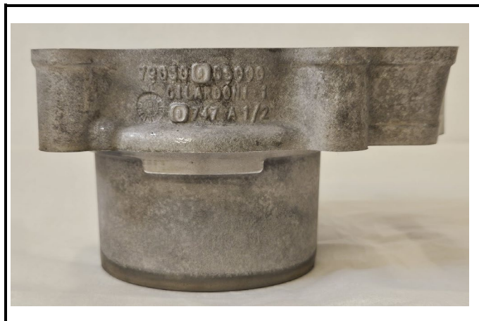
C3-16 Sylindrblokk sett fra innsugsiden Bare cylinder block seen from intake side
