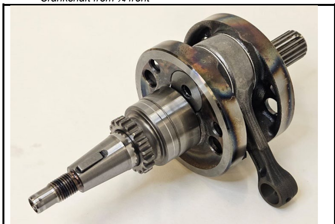
C6-1) Veivaksel sett \frac{3}{4} forfra Crankshaft from \frac{3}{4} front
