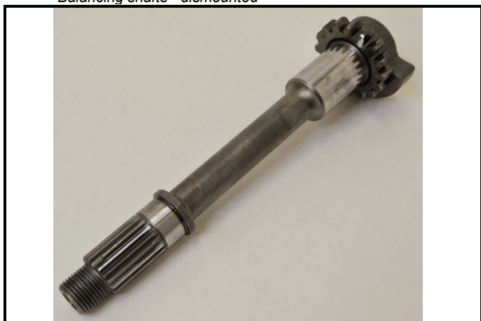
C3-9) Balanseaksel demontert Balancing shafts - dismantled
