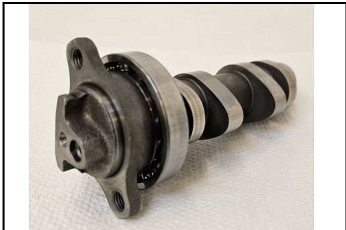
C10-5) Kammakselhjul - demontert Camshafts gears – dismantled
