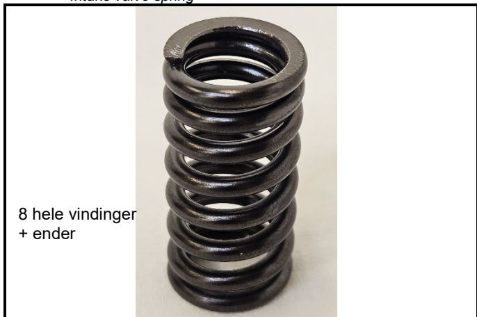
C10-8) Ventilfjær innsug Intake valve spring
