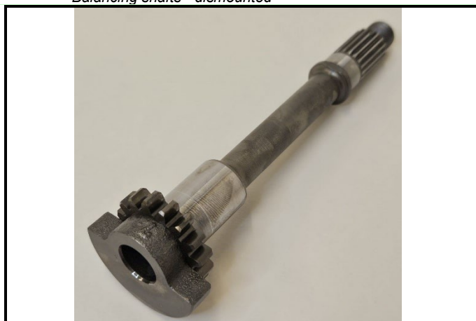
C3-10) Balanseaksel demontert Balancing shafts - dismantled
