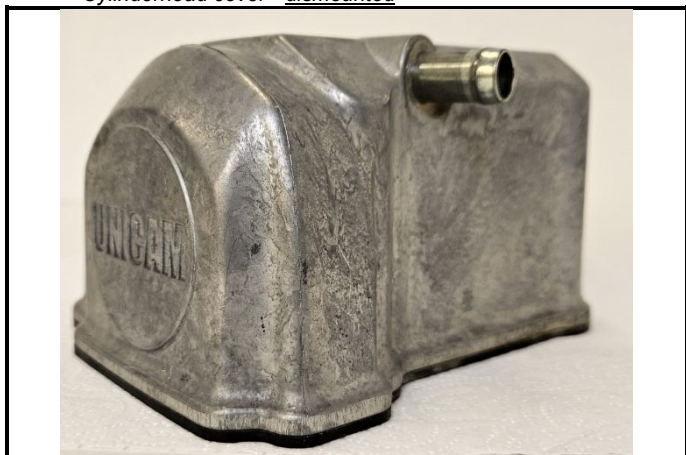
C1-3 Toppdeksel - demontert Cylinderhead cover - dismounted
