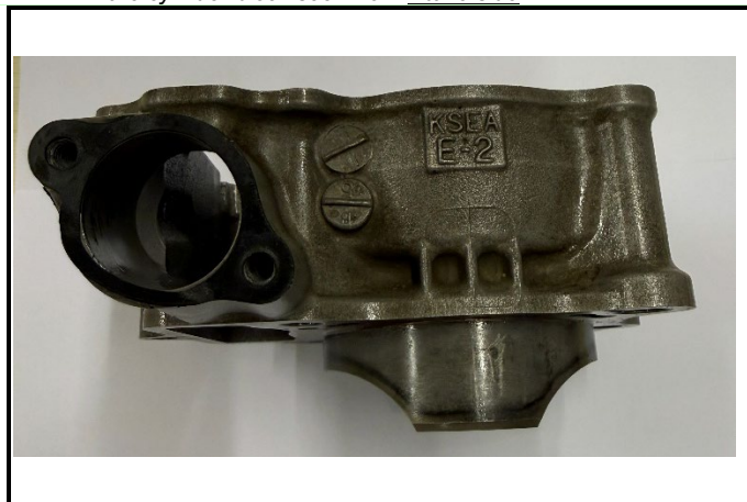
C3-16 Sylindereblokk sett fra innsugsiden Bare cylinder block seen from intake side
