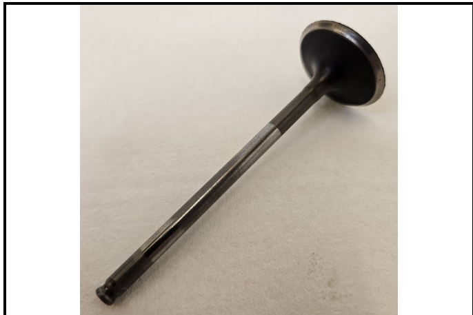
C11-5) Innsugsventil - demontert Intake valve - dismounted
