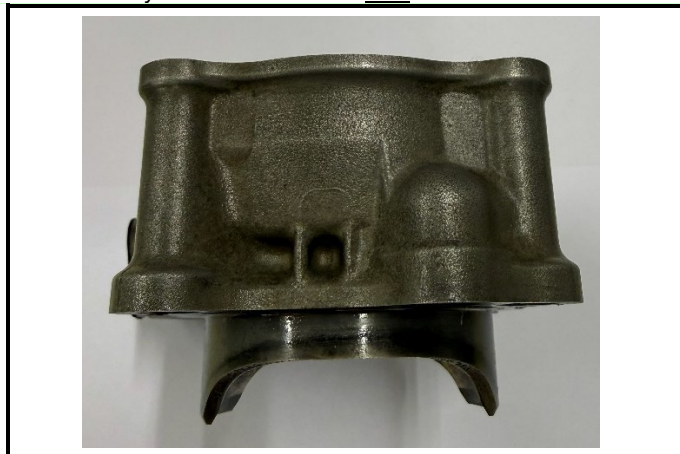
C3-16 Sylindereblokk sett fra innsugsiden Bare cylinder block seen from intake side
