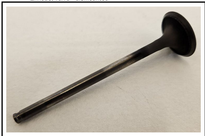
C12-1) Eksos ventil - demontert Exhaust valve - dismounted
