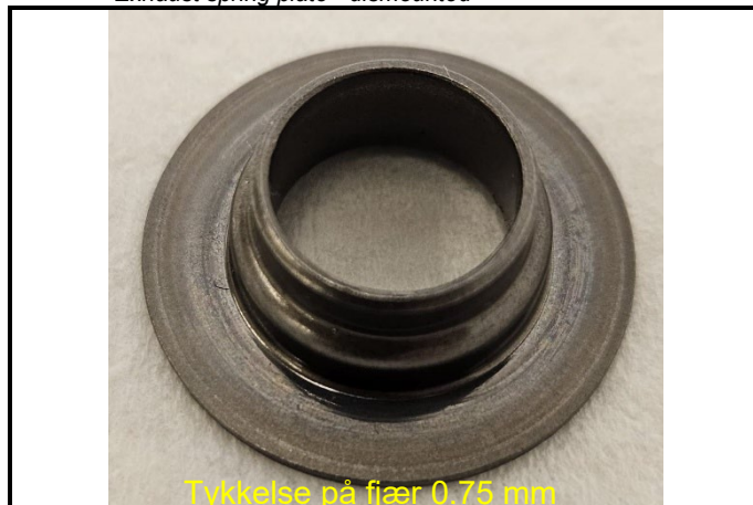
C12-2) Fjærplate eksosventil - demontert Exhaust spring plate - dismounted
