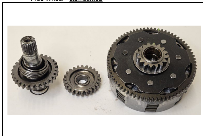
C16-2) Frihjul - demontert Free Wheel - dismounted
