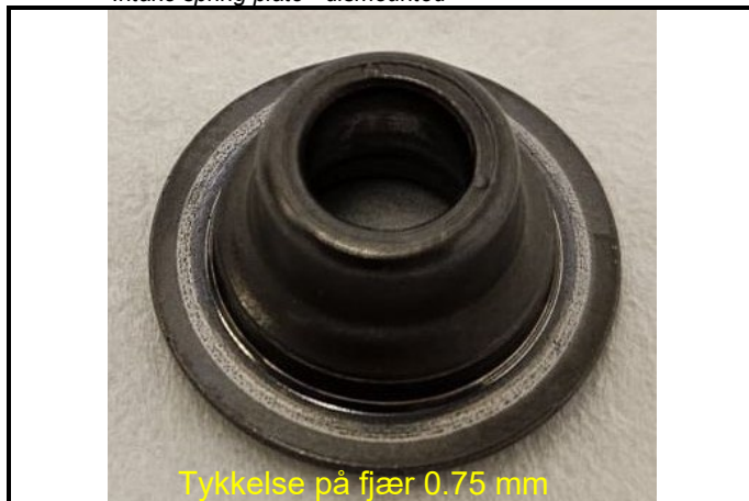
C11-6) Fjærplate innsugsventil bunn- demontert Intake spring plate - dismounted
