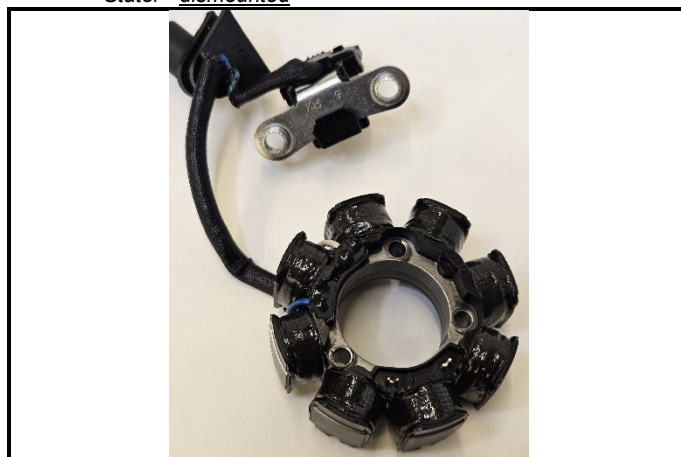
C15-2) Stator - demontert Stator - dismounted
